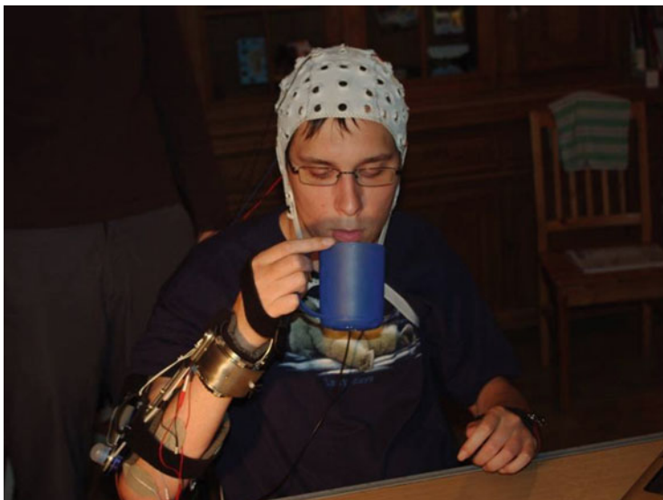
Fig. 7.3 A tetraplegic user holding a cup and drinking with the use of a BCI controlled FES hand and elbow orthosis
