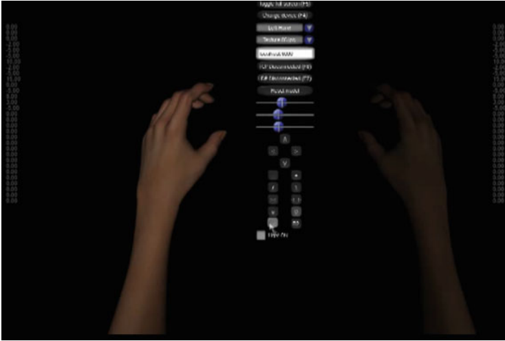
Fig. 7.5 Patient’s feedback is realized by means of a dedicated software which allows the therapist to reconstruct the image of the patient’s own hand, by adjusting size, appearance orientation, and other characteristics of the hand texture
