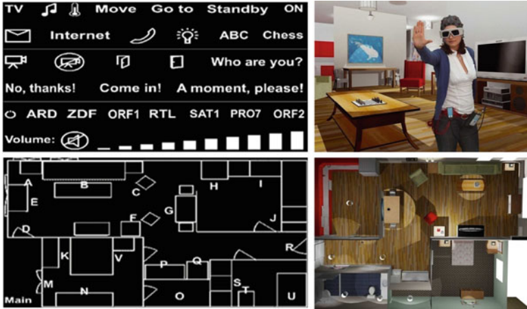
Fig. 10.8 Top left: Smart home control icons for TV, Telephone,... Top right: VR representation of the living room [15,29]. Bottom: Control icons to move to a certain position inside the apartment and corresponding bird eyes view of the apartment
