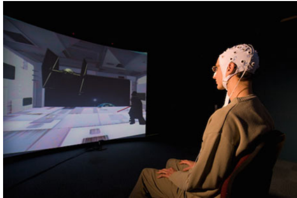
Fig. 10.4 The “Use-the-force” entertaining application [46], which enables its users to lift a virtual spaceship by using the BCI (© Hubert Raguët/Phototheque CNRS)
