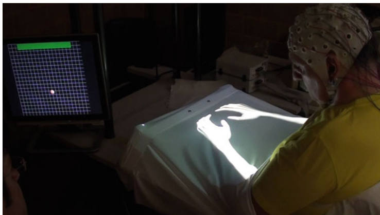
Fig. 7.4 Training session with the proposed BCI prototype currently under validation as an “add-on” rehabilitative intervention at the Fondazione Santa Lucia (Rome, Italy) within the TOBI project. The patient is trained to gain control of his visual hand representation by imaging hand movements (either closing or opening) and he receives as a feedback the congruent movements of the visual hand (successful trial). The therapist ( bottom, left corner ) is fed back with the real-time movement of a cursor on a screen that is actually controlled by the patient EEG relevant features
