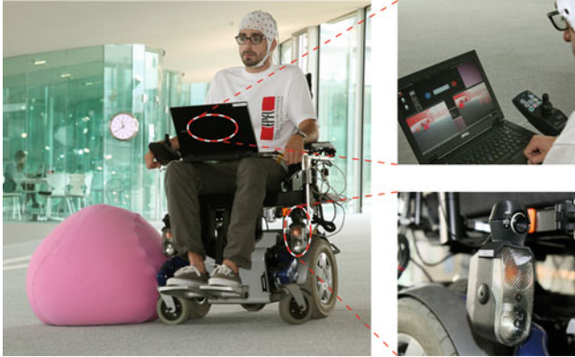
Fig. 6.3 Picture of a subject sitting in the BCI controlled wheelchair. On the right side two close-ups show ( below ) the webcams for obstacle detection and ( above ) the identified obstacles highlighted in red which will be avoided by the shared control
